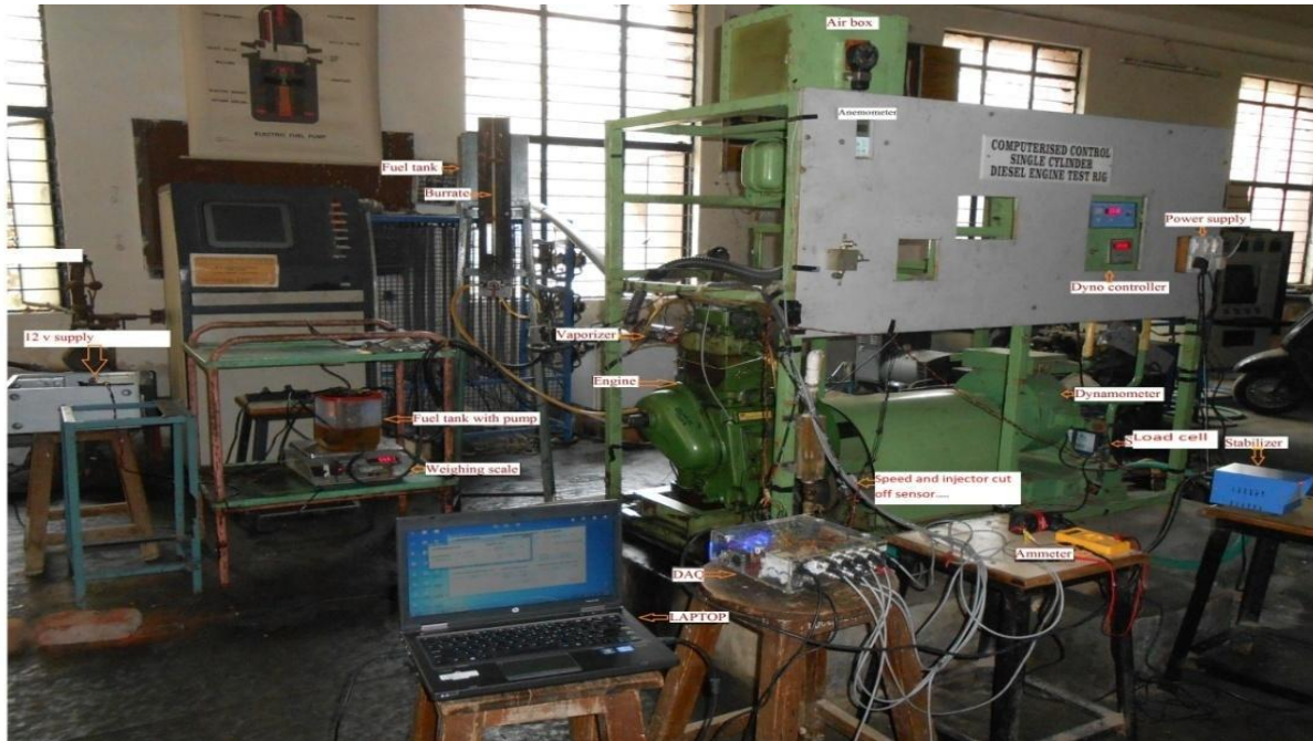
Fig 2.1 Actual experimental set-ups for modified engine (HCCI engine)
